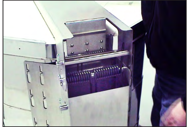
The properly Installed spring-hinge shown closed.
