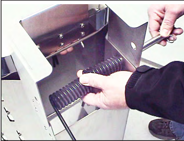
Removing the middle bar and springs.
