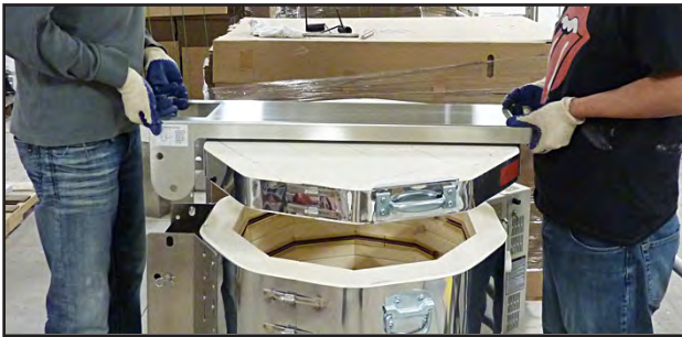
Lifting the lid off of the kiln body.
