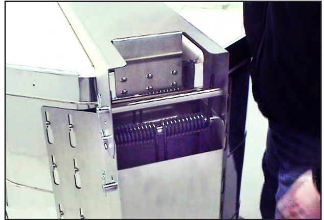
The properly Installed spring-hinge shown closed.
