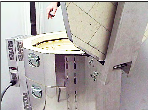
The properly Installed spring hinge open.
