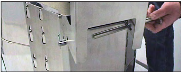
Installing the top-most rod.
