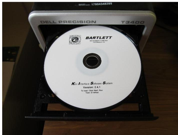
Insert the KISS CD in the computer's CD drive. If the CD does not automatically open, go to "My Computer" or "This PC" on your computer to find the CD Drive. Double click on the CD-ROM drive titled "(D:) KilnKISS 3.1. 2?". If it doesn't appear in the D: drive, select the appropriate drive. Open the file labeled "KISS" and double click "setup". Then, follow the on-screen instructions.
